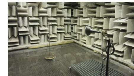
Acoustic development and testing in our own anechoic room in Malmö, Sweden
